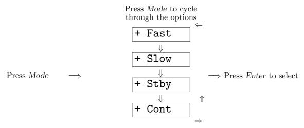
Having selected the required mode of operation, and pressing *Enter*, the HDI returns to the normal mode of operation, working in the newly selected mode.
